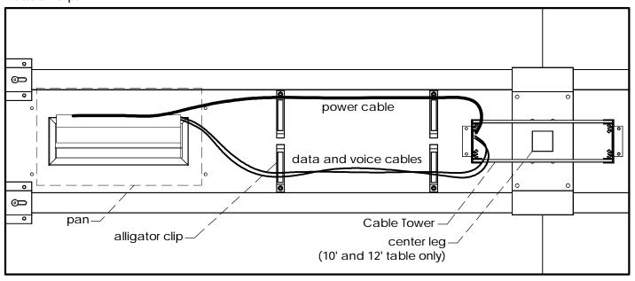
**Step 6**Route cables through Cable Tower (see Cable Tower instructions).
