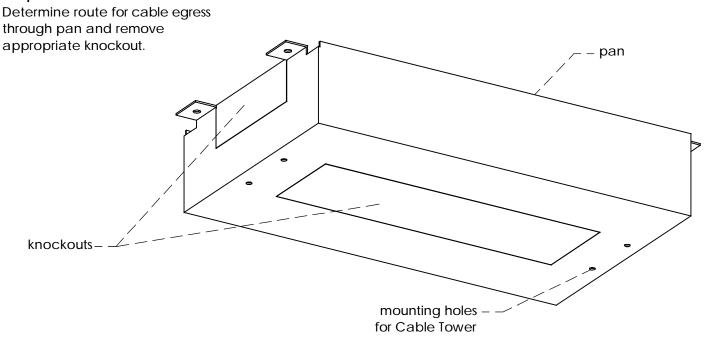
Step 4 Install pan under 5-3 Drop-in using #10 x 3/4" wood screws (FIG-1).
