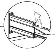
Step 1: For 15" wide drawers To remove top drawer, press plastic levers up or down on sides of drawer slides to disengage drawer.
