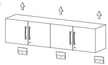
Step 2 Remove screws from steel cleats on wall.
