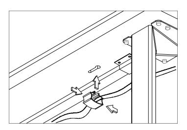
Step 2 Pinch sides of Snap inward and insert into key-hole slot on underside of desk.
